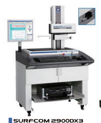
The detector is equipped with the device for measuring the surface roughness and high accuracy contour profile.
